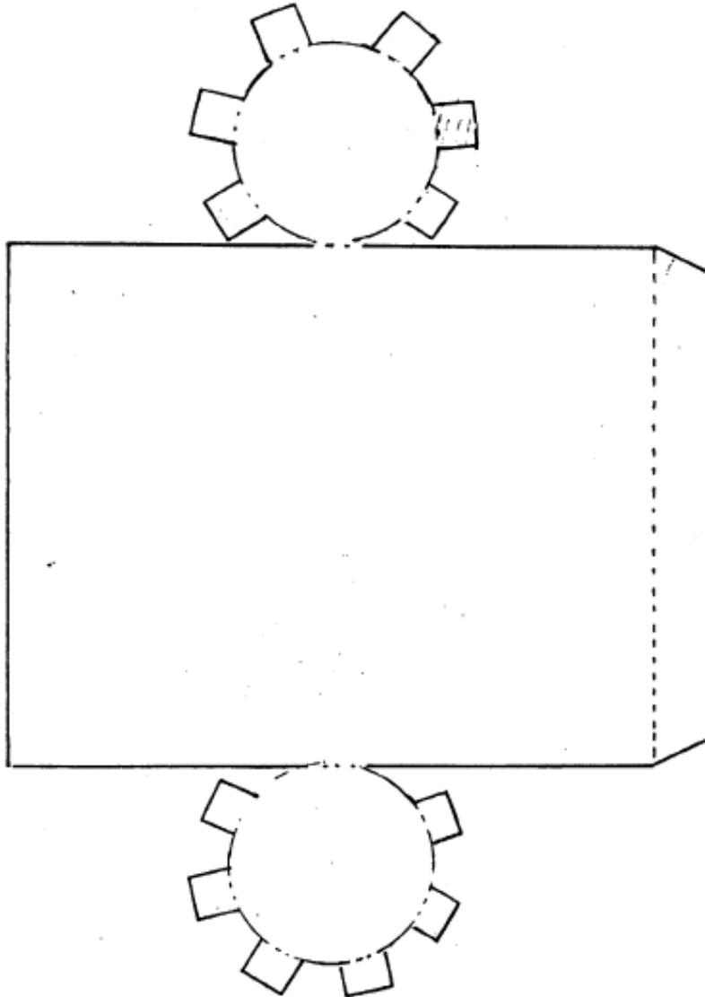
2. Fold the shape along the dashed lines. Form a cylinder like the one shown at right.
